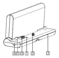
1 DC IN connector Connect the power adapter to recharge.
